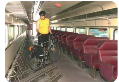
Racks on Transit
